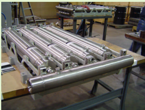
Low pressure, SS dryers, 400 SCFM
