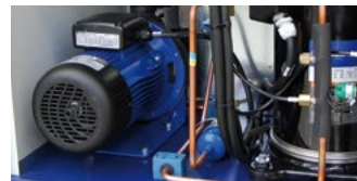
Pump P3 (3 barg) / P5 pump (5 barg, optional).
