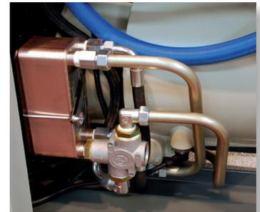
The "Heat Recovery" kit is totally integrated into the oil cooling circuit, making the unit independent from the oil temperature control and protected from any possible malfunctions, such as water flow reduction and overheating.
