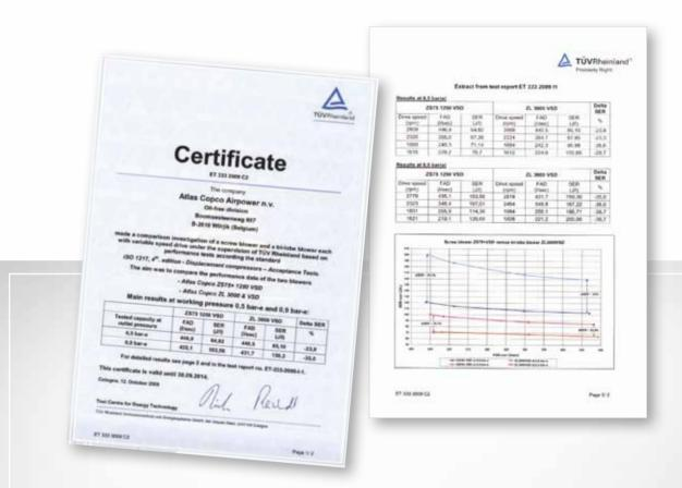
It was proven that the ZS+VSD is **23,8 percent more energy efficient** than a tri-lobe blower at 0,5 bar(e)/7 psig, and **39,7 percent** at 0,9 bar(e)/13 psig. The world-class efficiency of the ZS is mainly attributed to the superior screw technology.
