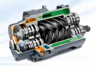
Efficient shaft sealing design of the oil-free blower element eliminates the risk of oil leakage and guarantees 100% oil-free air. We have triple safety barriers to prevent any oil to enter into the blower chamber:
